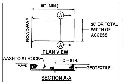
MAINTENANCE: Rock Construction Entrance thickness shall be constantly maintained to the specified dimensions by adding rock. A stockpile shall be maintained on site for this purpose. At the end of each construction day, all sediment deposited on paved roadways shall be removed and returned to the construction site. Note: AASHTO #1 Rock is equivalent to 3-4" rock.
